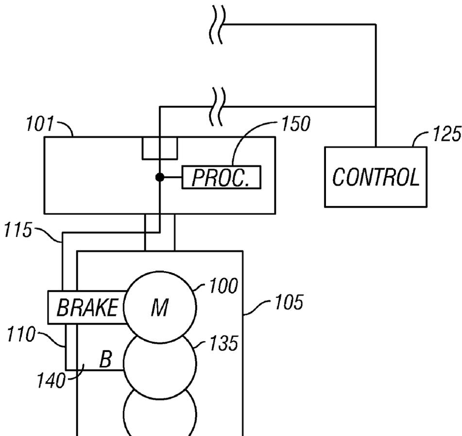
**PAN AND TILT SERVOMOTOR WITH BRAKE**
