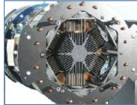
Fig. 7: Heat sinks and fans
