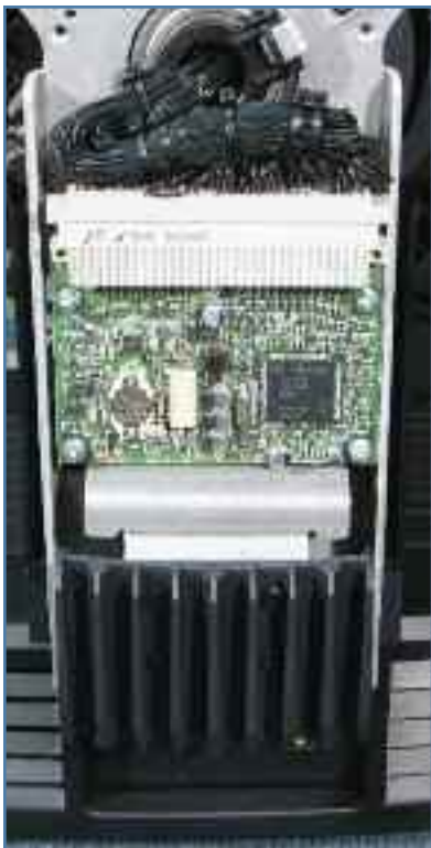
Figure 17 - Main control electronics
