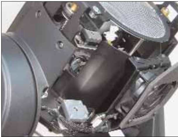
Fig. 13: Condenser and compound lenses
