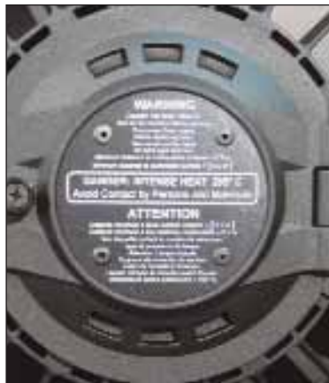
Fig. 3: Lamp replacement panel
