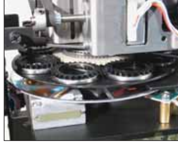
Fig. 12: Rotating gobo wheel.
