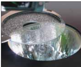
Fig. 5: Uniform field lens.
