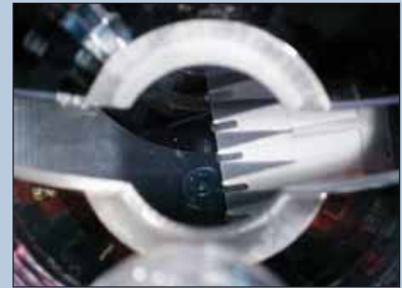
Fig. 3: Dimmer flag showing frost glass
